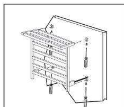
STEP7 Fix on the wall
