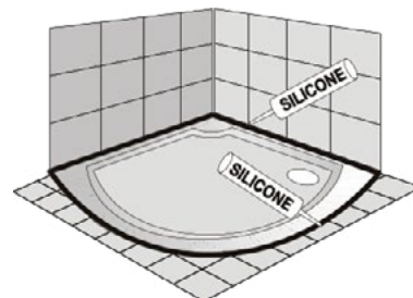
Recessed in the floor
